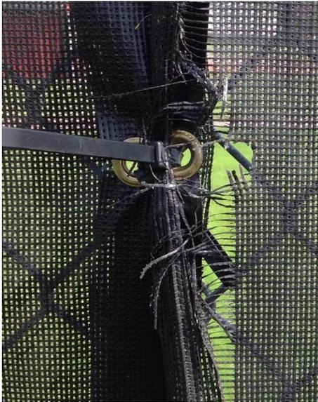
**Do not double-up the tie-wraps.** Each grommet should get it's own tie. Doubling up puts added stress on the grommets and fabric and will pull the hem or grommet out, as something has to give. When grommets are doubled up, the windscreen warranty is void.
